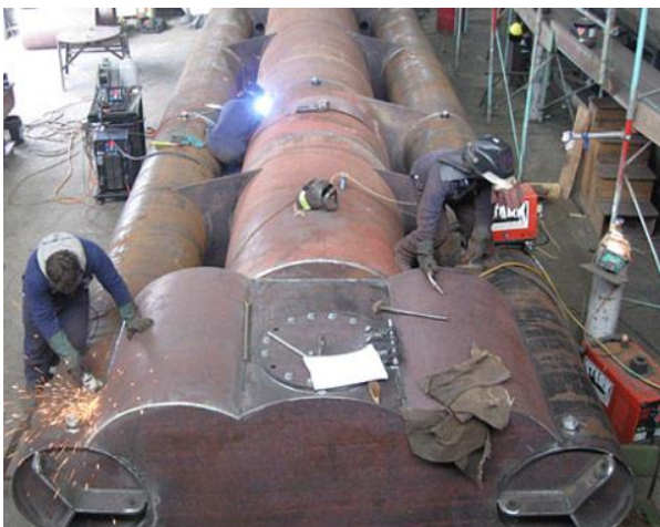
WET-NZ's - a research collaboration between IRL and Power Projects Ltd – half-scale wave energy device being fabricated at Stark Brothers in Lyttleton and being deployed for first sea trials
