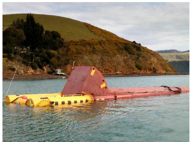
WET-NZ's - a research collaboration between IRL and Power Projects Ltd – half-scale wave energy device being fabricated at Stark Brothers in Lyttleton and being deployed for first sea trials
